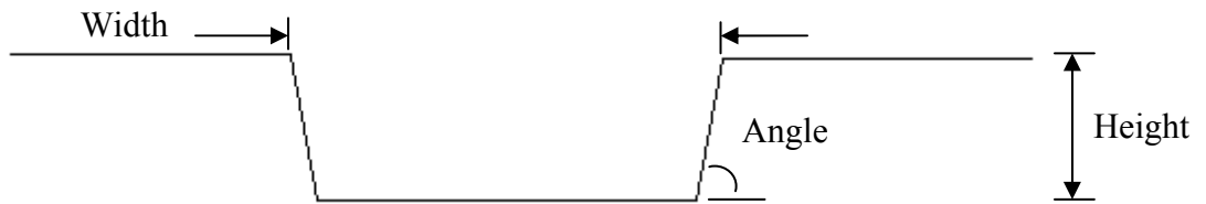
Figure 31 Sketch to show how dimensions were measured from printed pattern.
